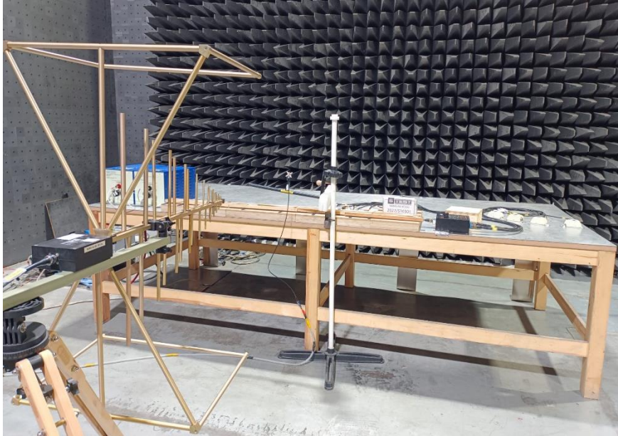
Resim 19: RS103 30-200MHz Dikey Test Kurulumu / Picture 19: RS103 30-200MHz Vertical Test Setup
